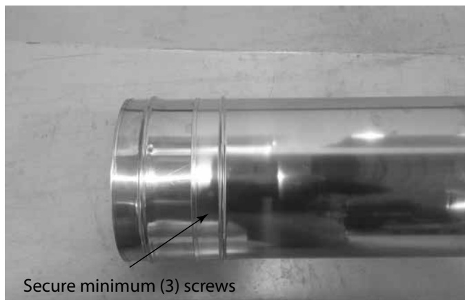
Figure 7.5 Screws into Slip Section
