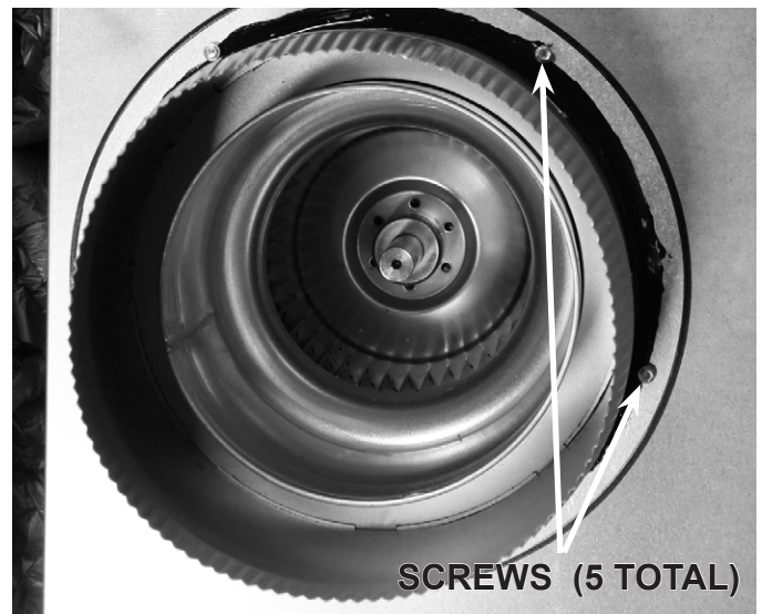
Figure 8F.4 Base Plate Fastened to Intake
