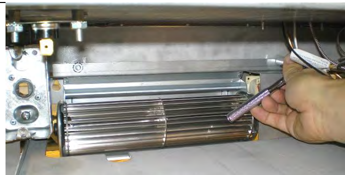
3. Hook Fan onto Studs. Replace and tighten nuts
