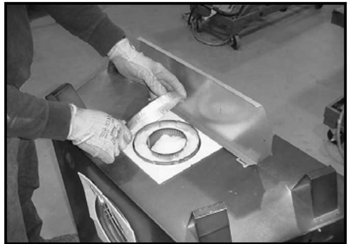
Figure 6.8 Remove the seal cap.
