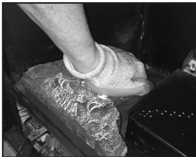
Figure 11.1 Press Left Hearth Firmly Into Place
