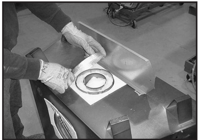
Figure 6.4 Remove the seal cap.
