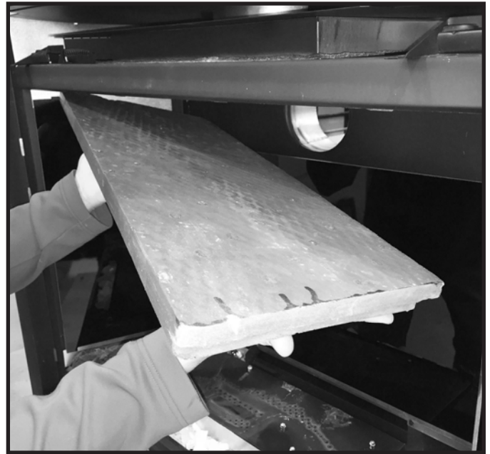
Figure 11.16 Install Top Refractory Panel
