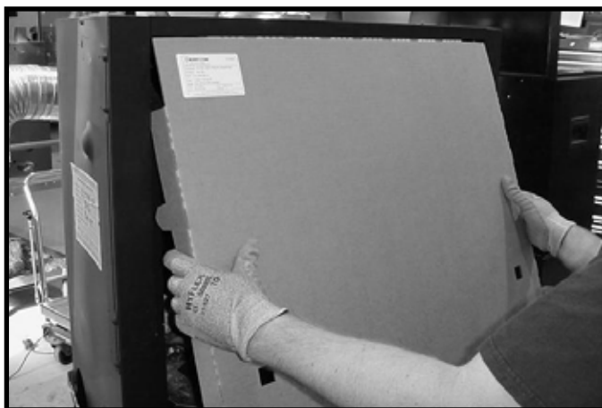
Figure 11.4 Installation of Splatter Guard
