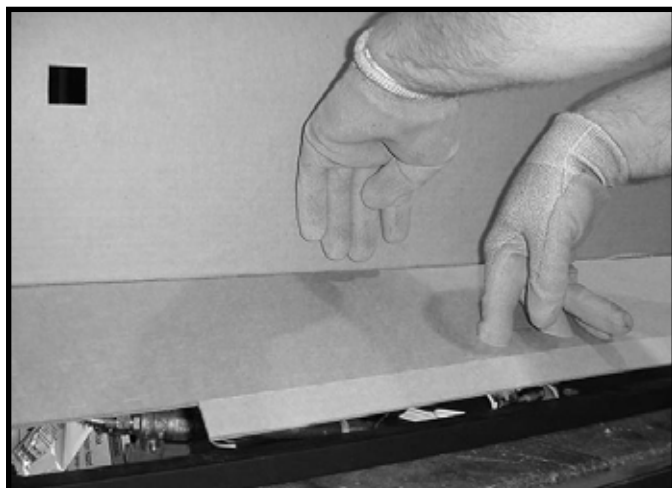
Figure 11.8 Opening Lower Access Panel
