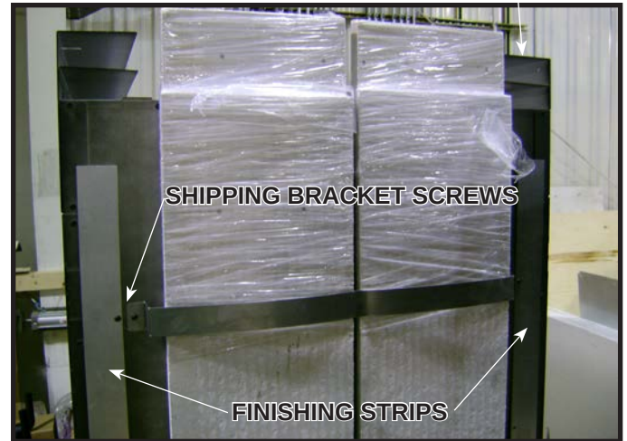
Figure 6.3 Shipping Brackets and Finishing Strip Locations.
